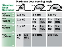
This guide is for standard butt hinged doors as shown in the diagram.
