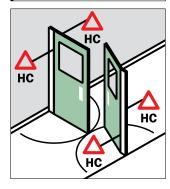
Pivot hinge doors with opening unrestricted up to  $180^{\circ}$  (Typically corridor doors).
