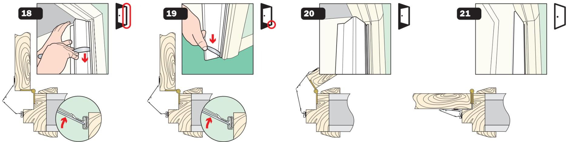
**Extending Door Finger Protector® shield section for doors opening beyond the span of one hinge shield section**
