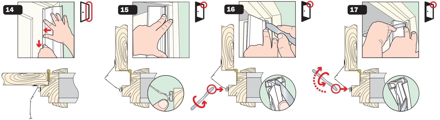
To temporarily unclip the shield for hinge access or door removal reverse stages 17 and 16 sliding knife downwards.
